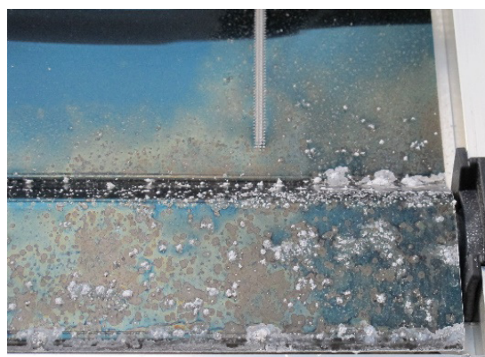
Figure 1: Salt deposition and corrosive degradation of the absorber layer near a pipe
